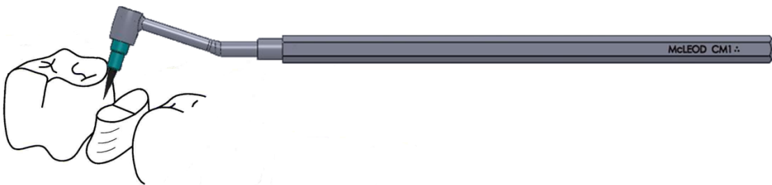
Figure 3. Marking the contact with the CM1
